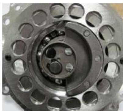
图 5-4 涡旋式膨胀机偏心轮 Figure 5-4 Eccenter of Scroll Expander
