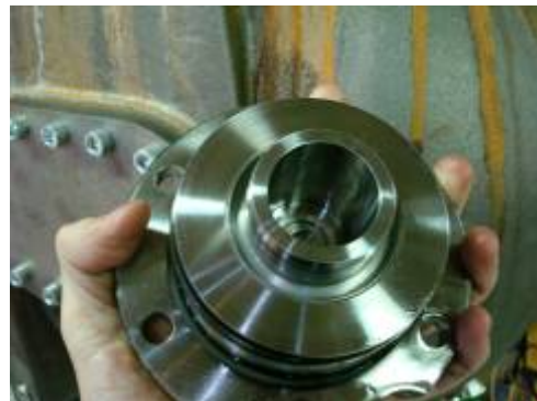
Removal of the filter housing cover
