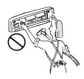
Do not put a stove, etc. where is exposed to direct air flow.
