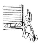
② Paste a heat shield film (generally available) on the window. Heat entering the room is reduced.
