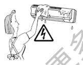
When an abnormality(smell of burning,etc)occurs,stop the air conditioner,and disconnect the power plug or turn off the breaker.
