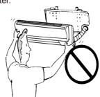
When the air filter is to be removed, do not touch the metal parts of indoor unit.
