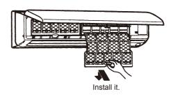
Function of the CATECHIN filfer: Along with the resolution of the CATECHIN (composition of green tea), the odour of cigarette and sweat is eliminated, furthermore the germ is restrainde to develop, grow up, and breed. (test method: Fiber product's quantitative germproof test method of Japanese textile inspection association.)
