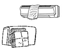
Check that the air inlet and outlet of the indoor/ outdoor unit are not blocked.
